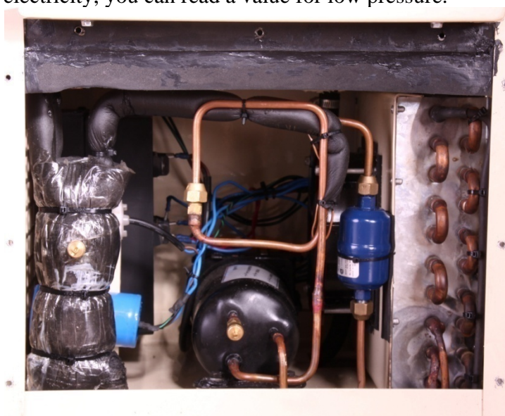
Figure 4- a view of bottom deck of refrigerator and its low and high pressure needles.
